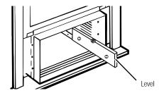
**NOTE:** When finished, use a level to make sure the case tilts to the outside 1/4" minimum. This prevents water from entering the room.
